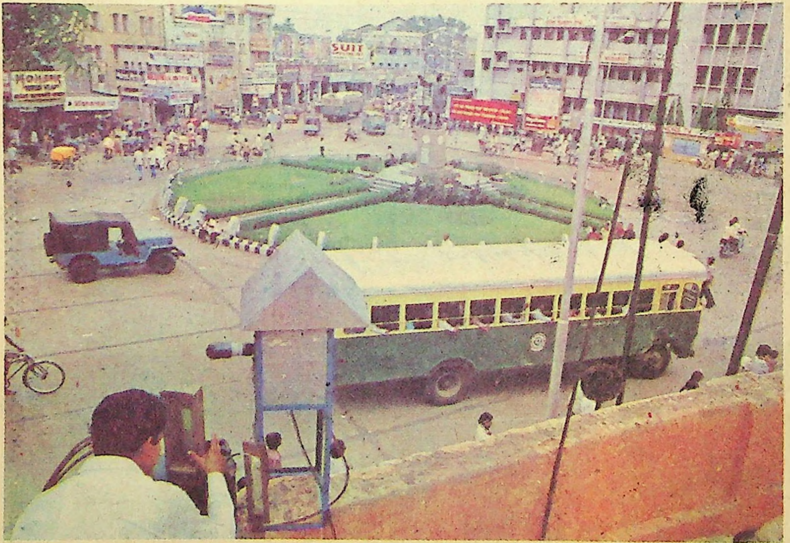
A Scientist measuring the presence of Gases entering the High Volume Sampler with the help of Manometer at Abid's Centre, Hyderabad, where the air pollution effects are found to be very high
