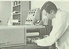
Above: The 34,000 gallon Electrocoat Primer tank, at the Castle Bromwich Works of Pressed Steel Fisher. The waterbased paint is topped up regularly with tanker loads delivered from Slough Works. Below: The 'Hardy' spectrophotometer and tristimulus computer enables an operator to make a permanent record of the colour of a paint in numerical terms. By using this apparatus, the operator can record colour differences which can only just be detected visually.
