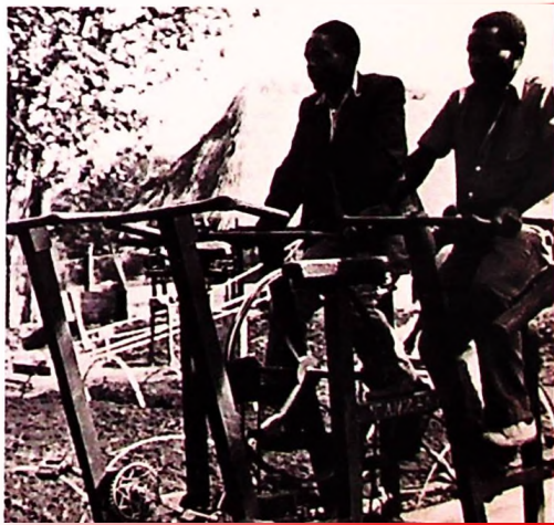
A two-man pedal-driven pump, constructed from locally available materials, raises water from below the surface to where it can be diverted into irrigation channels. (Photos WHO/UNICEF)
