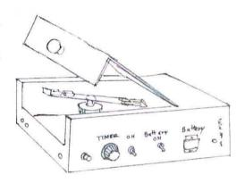
utilizes a portable capillary centrifuge (capifuge) and has been used extensively and found to be working reliably. The capifuge can run on AC mains or battery. The spin off advantage of this technique is the availability of the separated plasma which can be subjected to tests such as biochemical tests like that of glucose estimation!!
