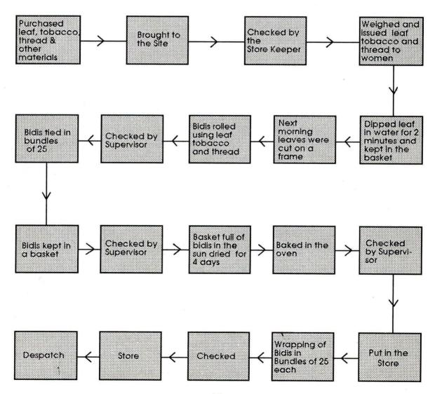
Such a process flow chart will help us estimate space, time, machines/tools and labour required at each step in a production-process. It will also explain to us the nature of linkages between different steps and their interdependence, etc.
