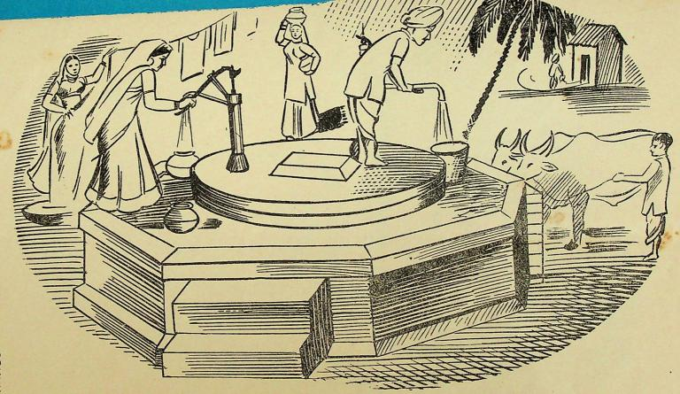
THIS IMPROVED WELL HAS A WATER-TIGHT LINING EXTENDING 10 FEET OR MORE BELOW GROUND. THE PUCCA TOP IS BUILT UP 2 FEET ABOVE GROUND AND HAS A WATER-TIGHT COVER. WATER IS DRAWN BY SANITARY HANDPUMPS RATHER THAN BUCKETS AND ROPES.
