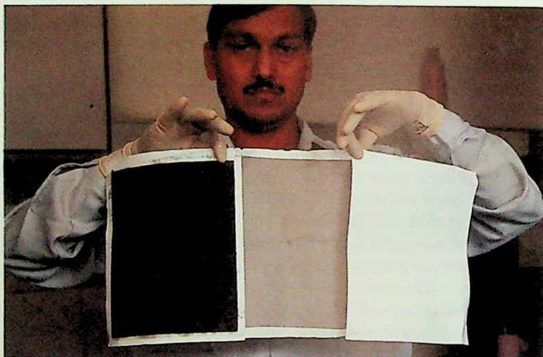
Figure 2 Pollutants turn a white filter paper to grey or black
